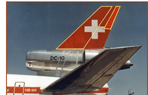
Douglas DC-10 composite Rudder and vertical stabilizer
